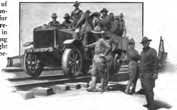
From the Popular Science Monthly THE TRUCKS EQUIPPED WITH THE FLANGED WHEELS CAN BE RUN OVER THE ORDINARY RAILROAD TRACKS OF STANDARD WIDTH
